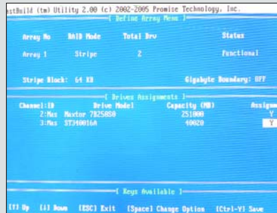
Access the RAID BIOS setup screen as soon as the system boots up
